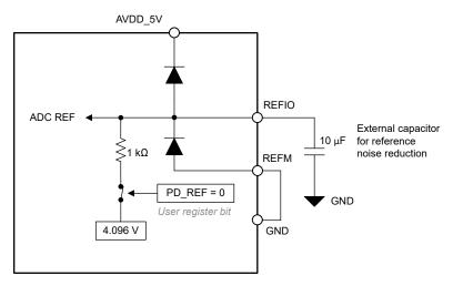
Figure 6-6. Internal Reference Voltage
