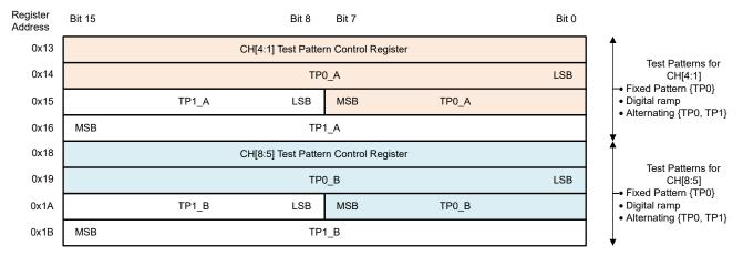
Figure 6-8. Register Bank for Test Patterns
