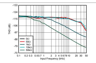
Figure 5-25. THD vs Input Signal Frequency Across Source Impedance With Wide-Bandwidth LPF, RANGE = ±10V
