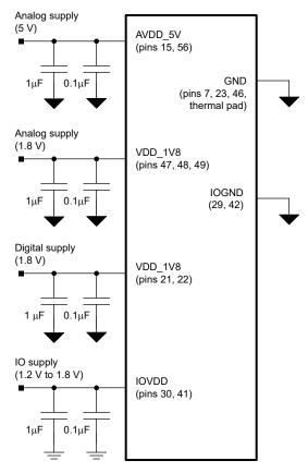
Figure 8-4. Power-Supply Decoupling
