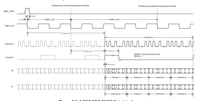
Figure 5-5. 2-SDO SDR CMOS Data Interface
