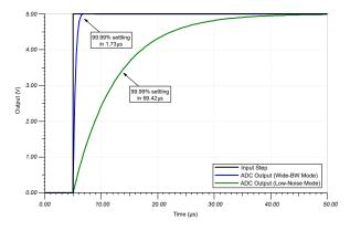
Figure 8-3. Step-Settling Performance
