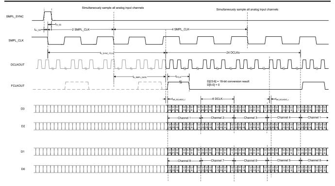
Figure 5-2. 4-SDO DDR CMOS Data Interface
