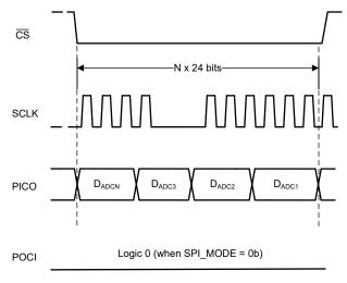
Figure 6-12. Register Write With Daisy-Chain
