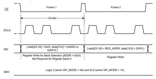
Figure 6-9. Register Write
