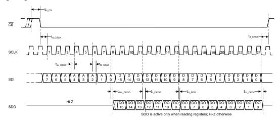
Figure 5-1. SPI Configuration Interface
