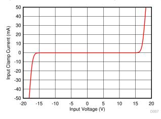
Figure 6-2. Input Protection Clamp Profile, Input Clamp Current vs Source Voltage
