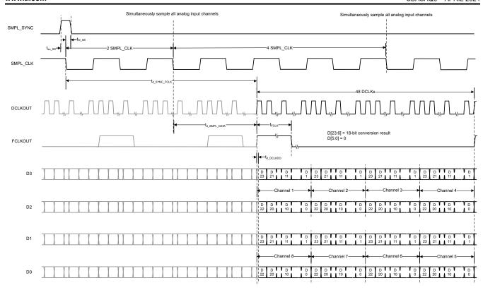
Figure 5-4. 4-SDO SDR CMOS Data Interface
