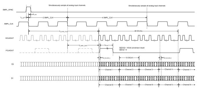
Figure 5-3. 2-SDO DDR CMOS Data Interface
