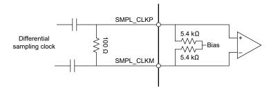
Figure 6-4. AC-Coupled Differential Sampling Clock
