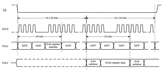
Figure 6-14. Register Read With Daisy-Chain
