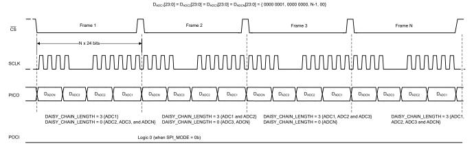
Figure 6-13. Register Write to Configure the Daisy-Chain Length
