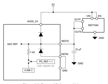
Figure 6-7. External Reference Voltage
