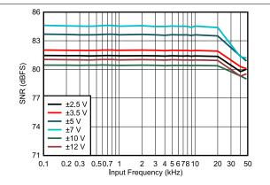
Figure 5-17. SNR vs Input Signal Frequency Across Input Ranges With Wide-Bandwidth LPF
