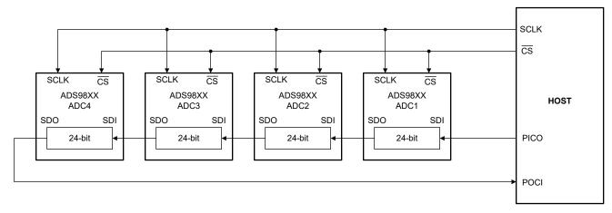
Figure 6-11. Daisy-Chain Connections for Configuration SPI
