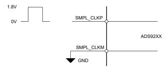
Figure 6-5. Single-Ended Sampling Clock
