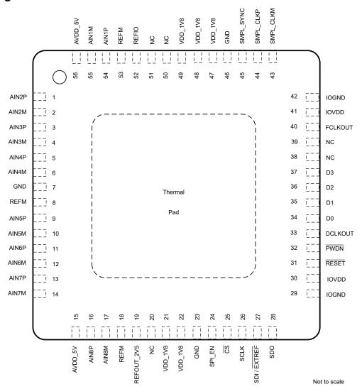
Figure 4-1. RSH Package, 56-Pin VQFN (Top View)
