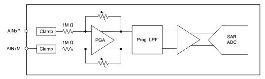
Figure 6-1. Front-End Circuit Schematic for the Selected Analog Input Channel
