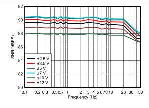
Figure 5-16. SNR vs Input Signal Frequency Across Input Ranges With Low-Bandwidth LPF
