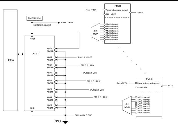
Figure 8-2. PMU With a Multiplexer
