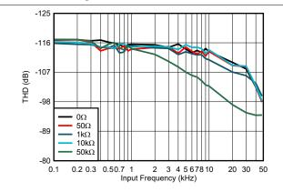
Figure 5-22. THD vs Input Signal Frequency Across Source Impedance With Low-Bandwidth LPF, RANGE = ±5V
