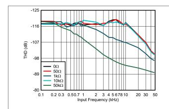
Figure 5-24. THD vs Input Signal Frequency Across Source Impedance With Low-Bandwidth LPF, RANGE = ±10V
