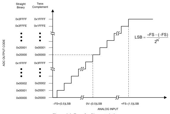
Figure 6-3. Transfer Characteristics
